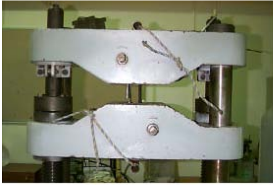
(a) The CIT tensile testing machine cross heads (b) Dial controls (The rope is to hold the pipe bollards in place when the specimen breaks)
