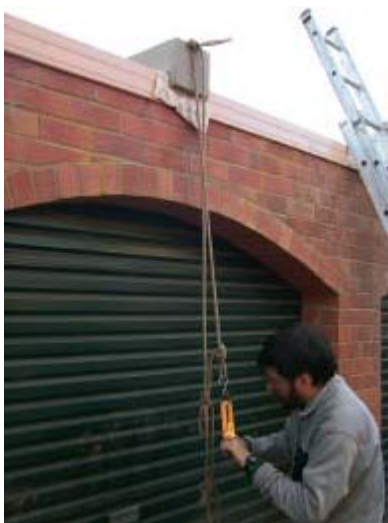
(a) The author using a spring balance to measure the load when pulling a knot over a 90° edge at his garage. the garage Figure 7 (b) The profile of the edges used for
