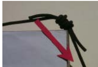
The Double Fisherman's Knot jamming on the edge. The arrow indicates the direction of pull.
