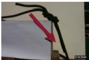
Figure 9 Rethreaded Figure 8 knot jamming Figure 10 Overhand knot clearing Knots
