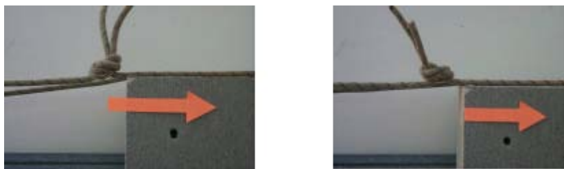
(a) Tails leading (b) Tails trailing Knot tails on the reverse edge. The arrow indicates the direction of pull. Figure 12
