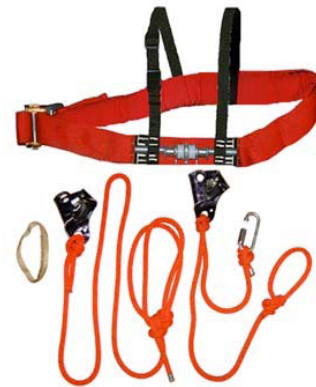
Figs 3 (left) and 4 (right): Double rope loops may be used in place of sewn stirrups for the Mitchell System. This decreases system weight and bulk and greatly facilitates the Frog conversion. Both loops go over the same foot when using the Mitchell and one loop on each foot for Frogging (Fig 3). The double foot loop requires a chicken loop when using the Mitchell. The short Mitchell ascender is not used in this configuration and can be stored until needed. Fig 4: A complete minimum weight (1200g) and bulk Mitchell System is shown at right.
