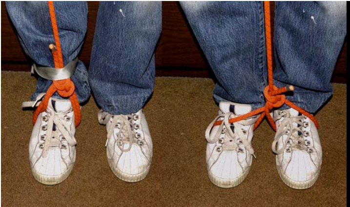
Figs 3 (left) and 4 (right): Double rope loops may be used in place of sewn stirrups for the Mitchell System. This decreases system weight and bulk and greatly facilitates the Frog conversion. Both loops go over the same foot when using the Mitchell and one loop on each foot for Frogging (Fig 3). The double foot loop requires a chicken loop when using the Mitchell. The short Mitchell ascender is not used in this configuration and can be stored until needed. Fig 4: A complete minimum weight (1200g) and bulk Mitchell System is shown at right.
