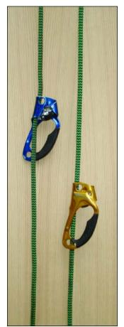
Figure 2. The left and right Petzl Ascension single-handled ascenders on the two legs of a doubled line.
