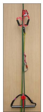
Figure 5. If a climber prefers the angled grip of the Kong Twin and still wants to use the lower Mar-Bar for his or her feet, the upper Mar-Bar can be easily exchanged for the Twin. Some type of backup system is recommended. Here the tether attached to the Twin is a Prusik loop with a webbing sling as an adjuster.
