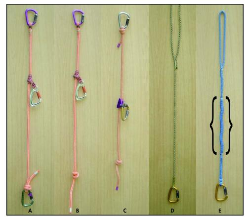
Figure 1. Five different types of tether setups, each of which uses a single length of line or cord. Because these tethers use only a single piece of line rather than a doubled line, the line must have a minimum tensile strength of 5,400 pounds.
