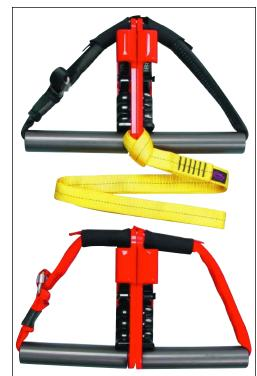
Figure 4. Mar-Bars use two single-handled CMI Ultracenders to form a single, double-handled upper ascender (with yellow strap) for the hands and two more Ultracenders to form a single lower ascender for the feet. The climber is attached to the upper ascender only and uses the lower ascender simply to assist in his or her inch-worm progression to the top. Because the climber is attached only to the upper Mar-Bar, it is recommended that another system be used as a backup.
