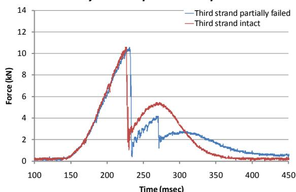
all of the failures showed the multiple peaks on the force/time plot characteristic of uneven load sharing. Two of the four polyester samples failed on the first drop, with the remainder failing on the second. Both of the first drop failures exhibited the symptoms of uneven load sharing. Both of the
