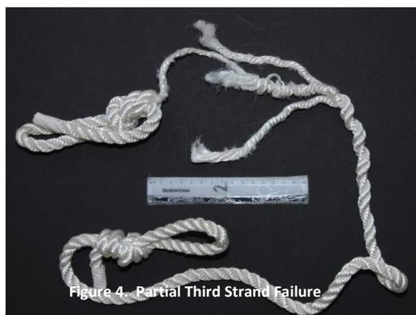
Figure 4. Partial Third Strand Failure
