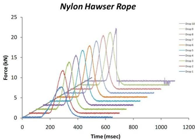
The results of the nylon hawser and nylon kernmantle tests are shown in Figures 5 and 6 respectively. A single sample was tested in both cases. The nylon hawser rope survived nine drops; the nylon kernmantle survived 26.
