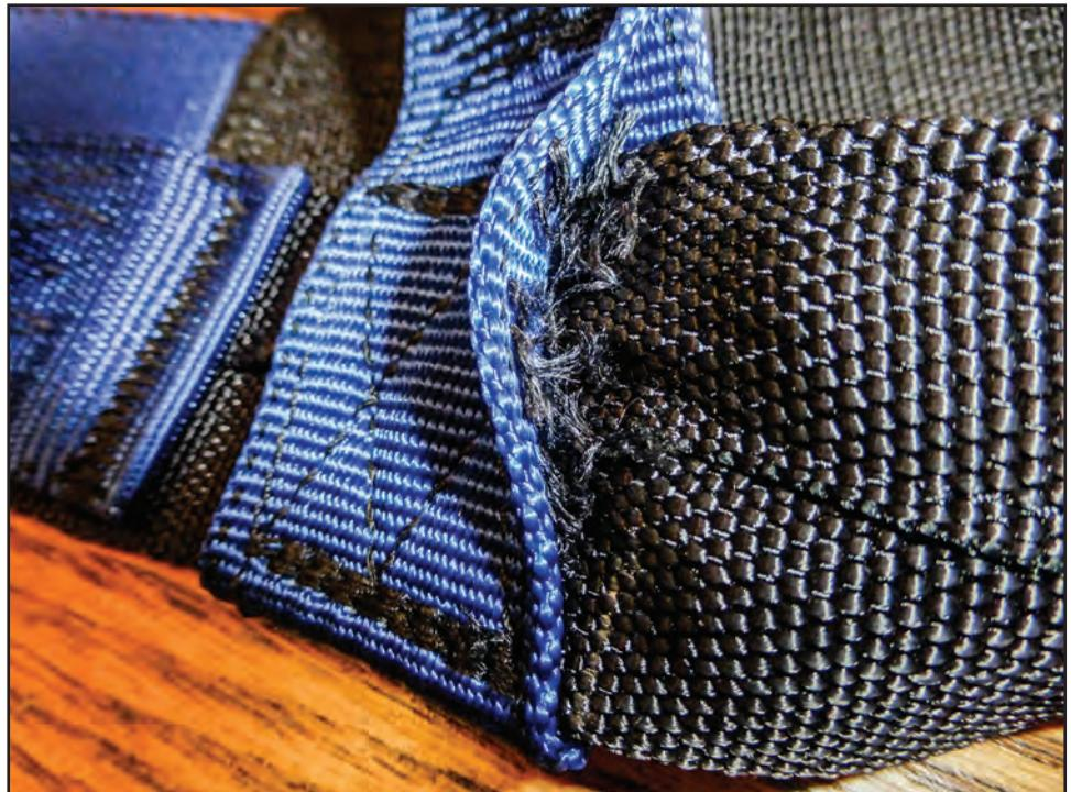
Figure 8—Some seam failures occurred during the 5,000 pound-force test.
