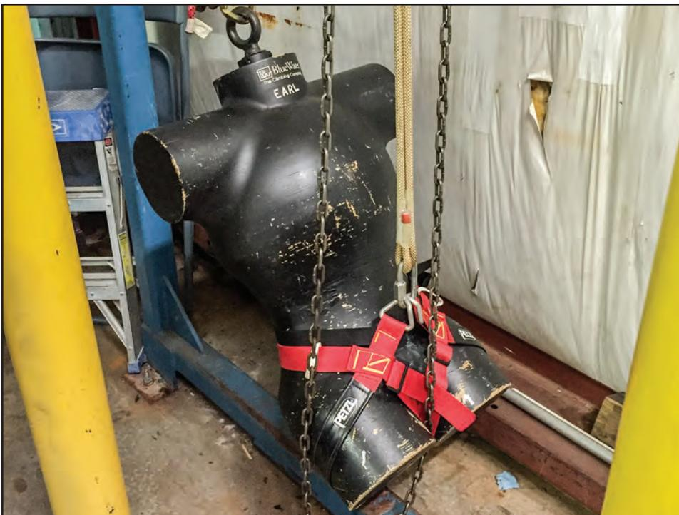
Figure 6—A dummy and test apparatus setup ready for a harness pull test.
