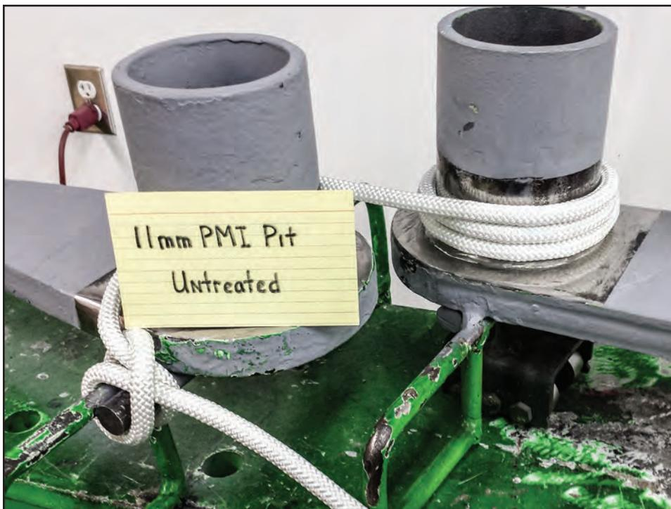
Figure 4—Holloway Houston, Inc., pull-tested rope samples until the samples broke.
