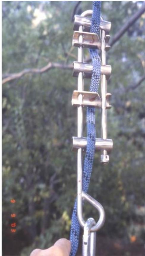
For our testing we removed the 6<sup>th</sup> bar completely from the rack, so it could not interfere in any way with the test. We would release the test mass from varying heights, which would give different lengths of rope between the belayer and the rappeller and different lengths of rope between the rappeller and the anchor.
