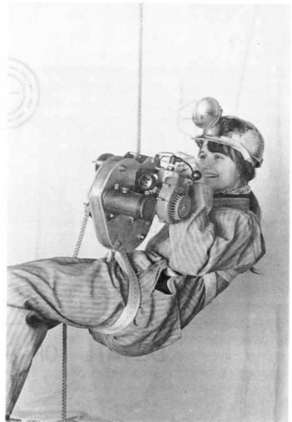
Figure #10 This illustrates the use of a modified MAD in ascending, Note that the climber is secured with a seat sling and an auxiliary sling around the chest to hold her vertical, Both the throttle and stop controls are operated with the left hand,
