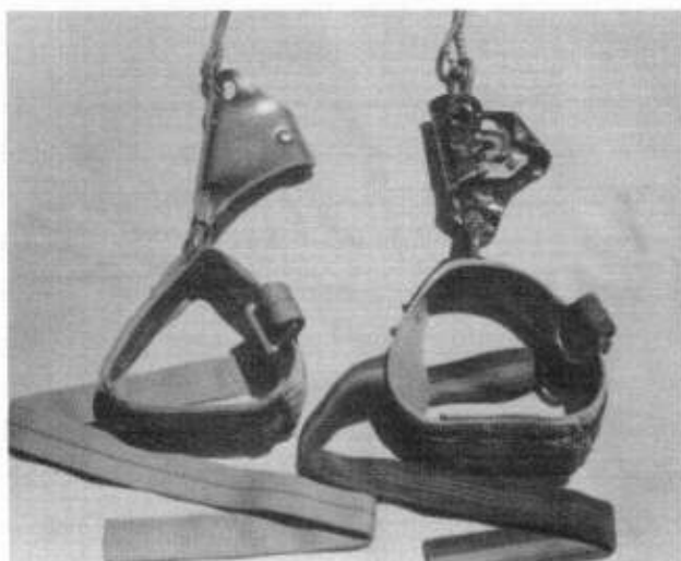
Two foot loops from 2 rigs. The left one uses a #3 Maillon to connect bungee cord, while the other uses a pear shaped snaplink.
