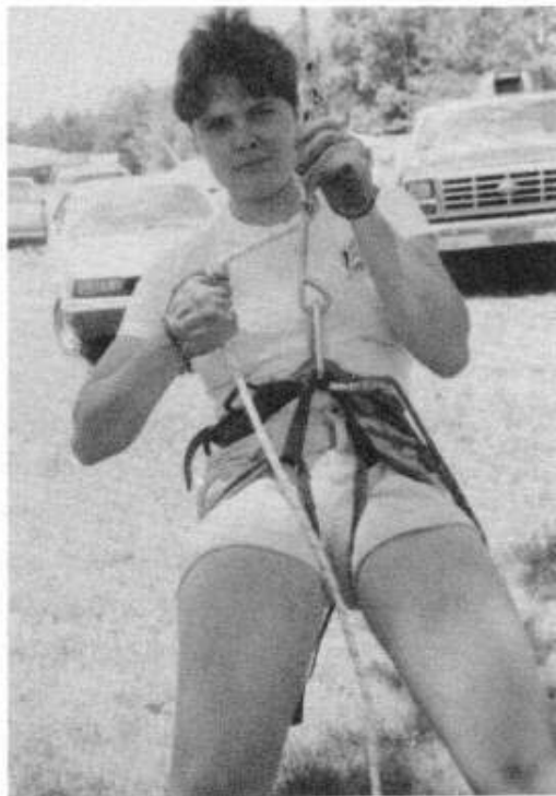
A twisted eye rack properly oriented.
