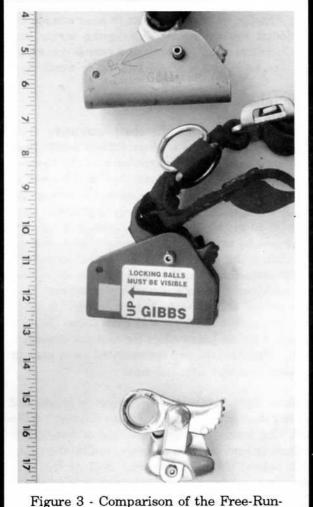
Figure 3 - Comparison of the Free-Running Gibbs, the Hinged Gibbs and the G.O.S.H Cam
