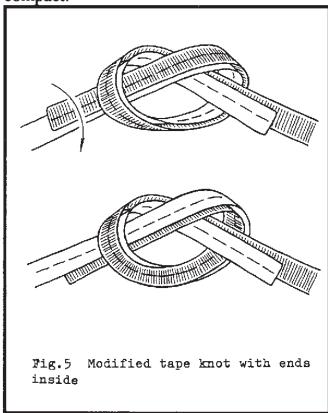
The strength wasn't the problem, but when the ends are inside, the standing parts are outside, where the radius is longer. This should be an advantage, and in fact the test of the author show the strength is increased.
